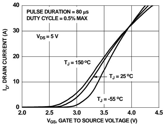
Figure 5. Transfer Characteristics
