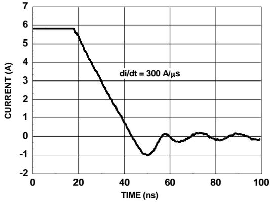
Figure 27. FDMC8200S SyncFET body diode reverse recovery characteristic
