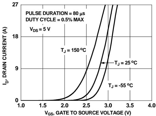
Figure 18. Transfer Characteristics
